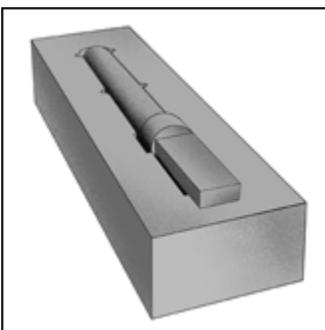
**3.** A sand core is made that fits precisely within the mould leaving a space between the core and the mould that will produce a constant and exact metal thickness.
