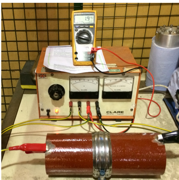
Electrical Continuity Testing
